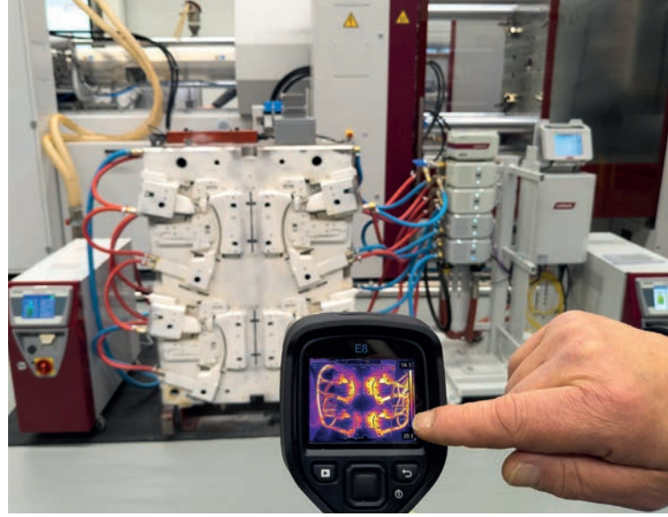
The stand-alone installation clearly illustrates the functionality. With Expert MouldTemp (right mold half), the heat distribution is very homogeneous. The faster heat-up can also be seen.
