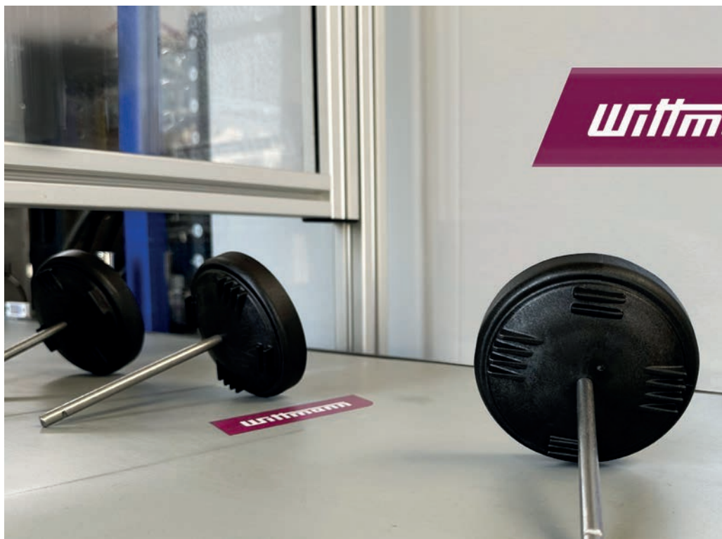
To produce the pressure vessel tops, the piston rods are directly over-molded. The material processed is fiberglass-reinforced polypropylene.
