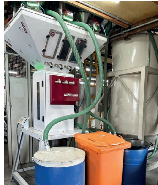
The new large Gravimax meters and mixes together up to six materials with extreme precision.
