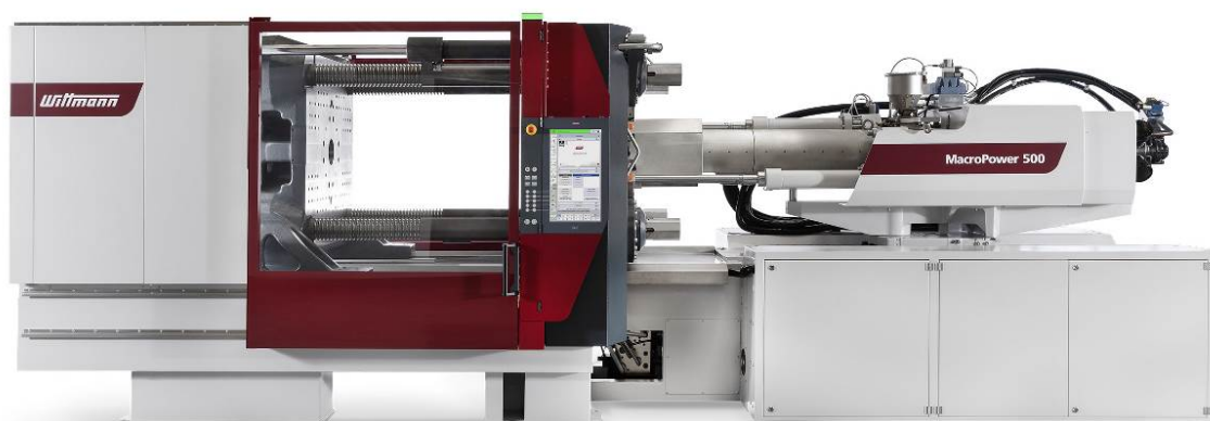
Fig. 1: MacroPower 500/3400 with one-piece machine body
