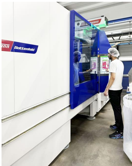
The control system integration of both the injection molding machine and the robot facilitates operation of the production cell.
