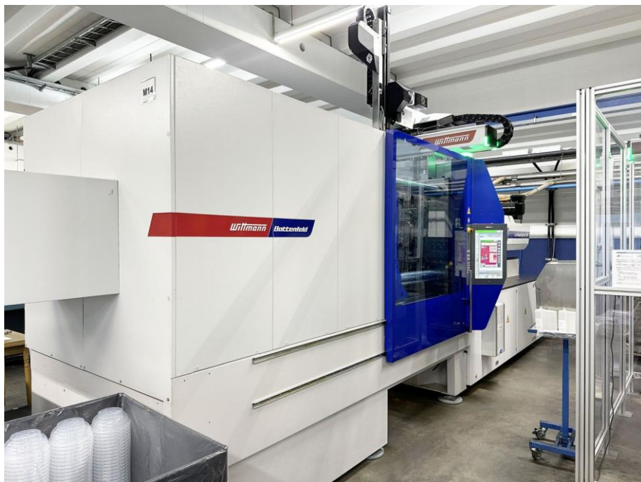
With the new EcoPower Xpress, Heinrich Axmann is entering the all-electric injection molding age.
