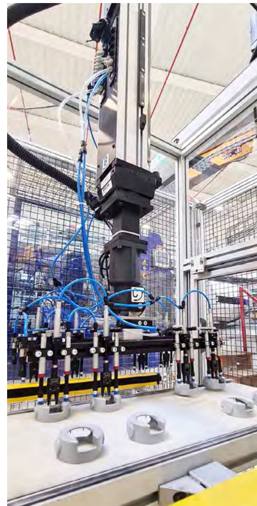
Views of cap handling actions on the conveyor belt within a secure environment.
