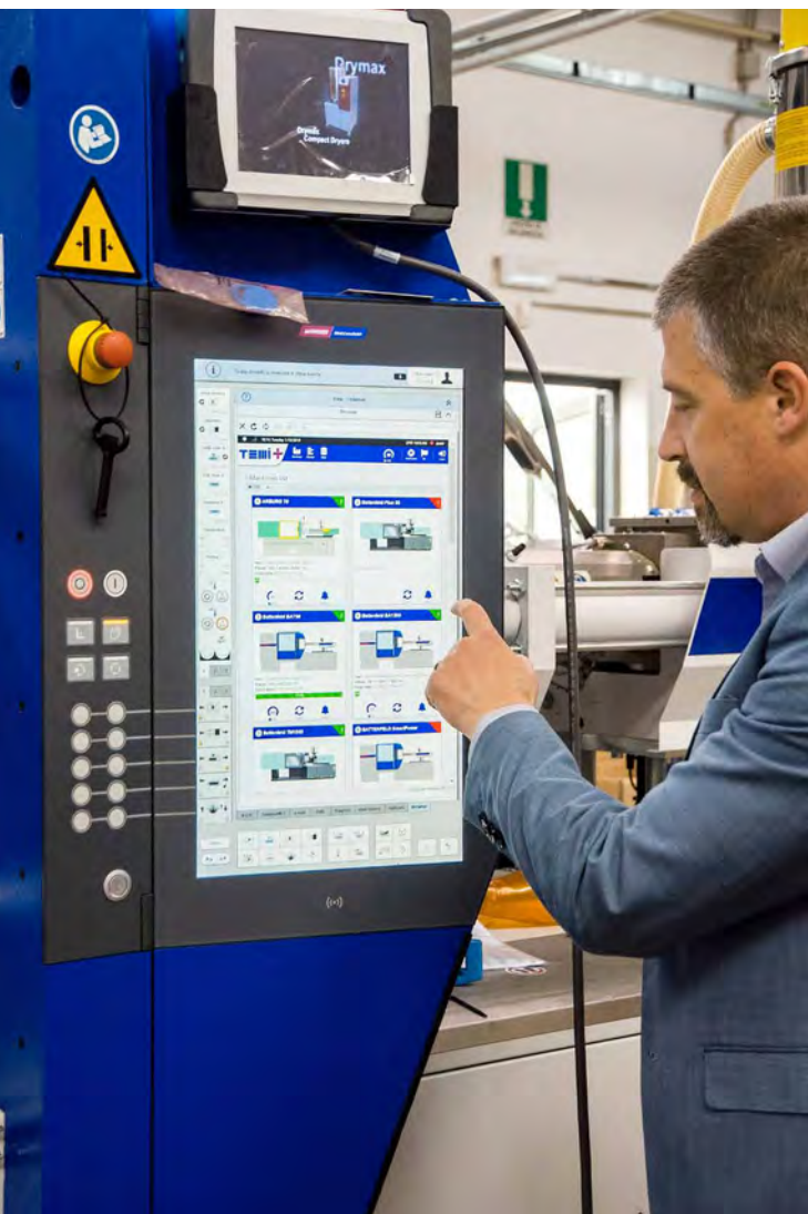
The MES system installed at the Stamplast plant in Belluno makes it possible to control the production process not only at the machine directly, but gives also remote access.
