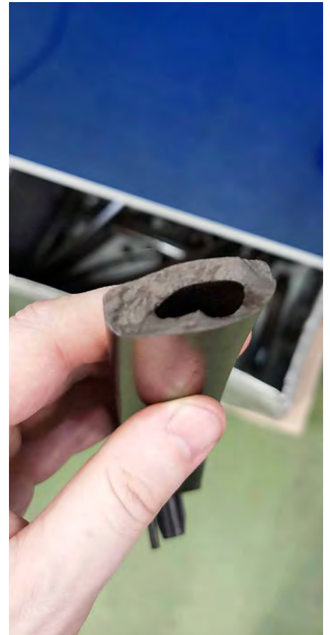
Domestic appliance door handles injection molded by GEFEST, applying the WITTMANN BATTENFELD AIRMOULD® technology.
