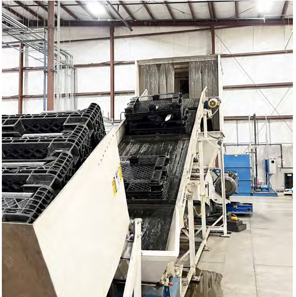
End-of-life plastic pallets being conveyed into granulator for processing.
