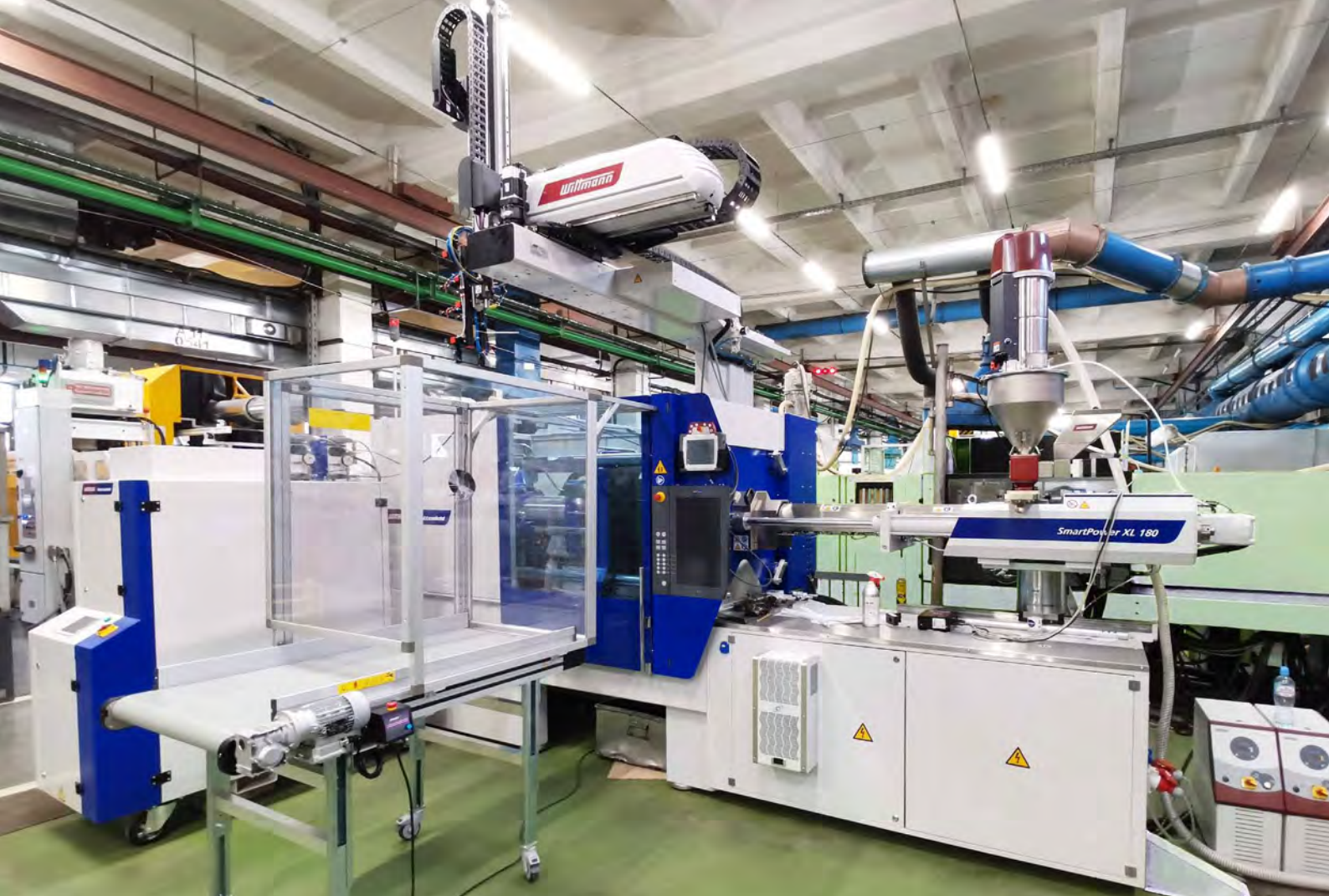
Views of a WITTMANN Group production cell at the GEFEST production plant in Brest, Belarus, consisting of a WITTMANN BATTENFELD SmartPower XL180 injection molding machine and a PRIMUS 26T robot from WITTMANN as well as different WITTMANN auxiliaries such as conveying equipment and temperature controllers.
