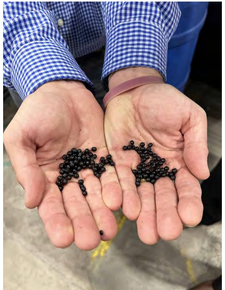
Reprocessed pellets made from the ground up tote plastic.
