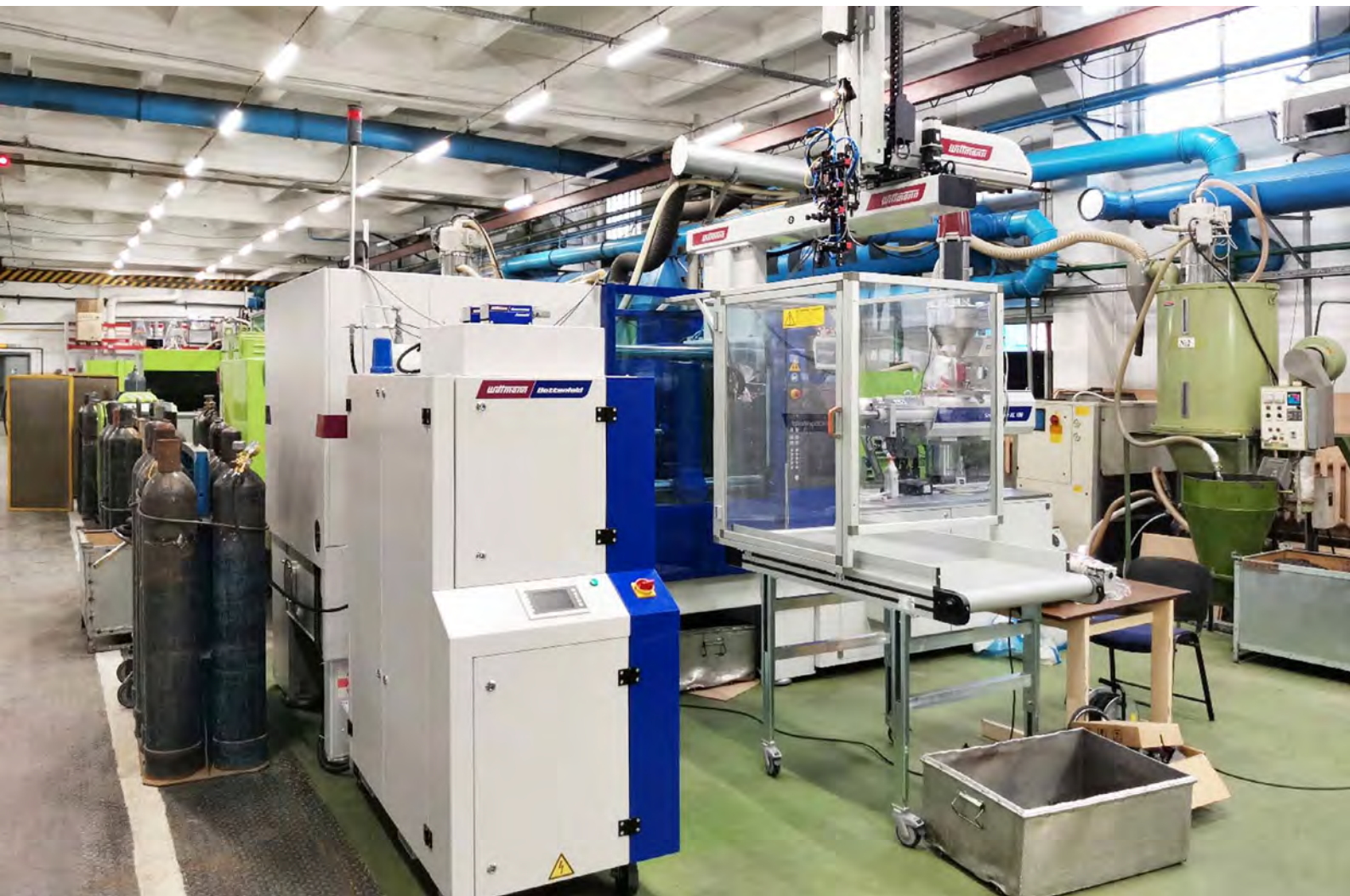
Views of a WITTMANN Group production cell at the GEFEST production plant in Brest, Belarus, consisting of a WITTMANN BATTENFELD SmartPower XL180 injection molding machine and a PRIMUS 26T robot from WITTMANN as well as different WITTMANN auxiliaries such as conveying equipment and temperature controllers.
