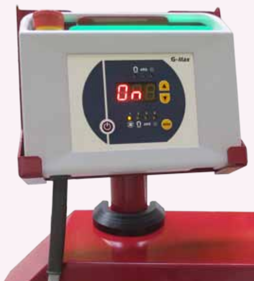
G-Max control with ambiLED visual status display
