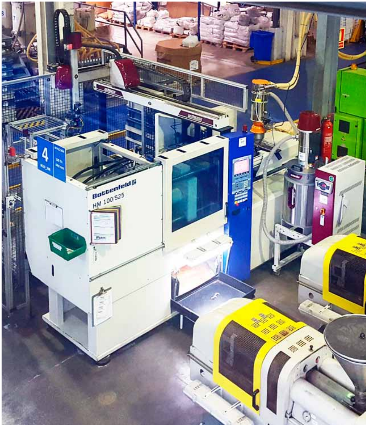
Hydraulic injection molding machine from WITTMANN BATTENFELD, and automation and drying equipment from WITTMANN at Simon in Olot.
