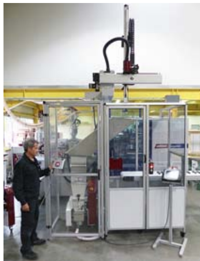
The G-Max 12 granulator is shown here within the protective housing of a working cell.
