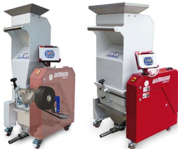
The G-Max 12 is the smallest model of the new series of beside-the-press granulators from WITTMANN, pictured here with drive visualization (left). G-Max 33 (right), the strongest model of the new granulator series.
