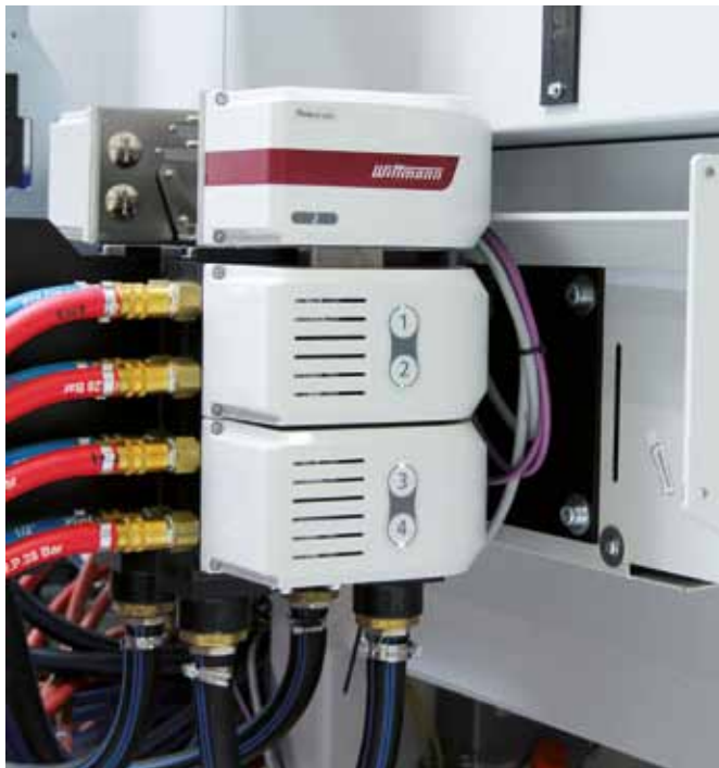
In operation at COLOP: The new FLOWCON plus from WITTmann improves temperature distribution in the mold.
