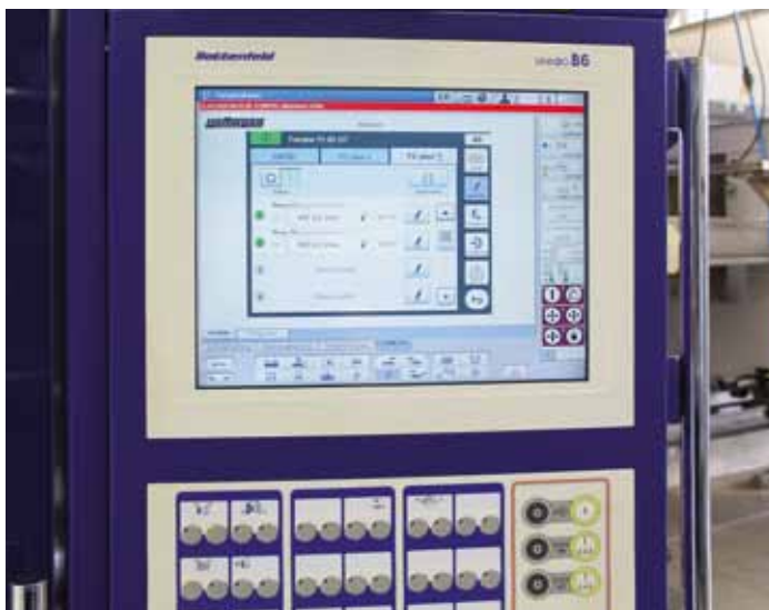
FLOWCON plus, integrated in the B6 P machine control system.
