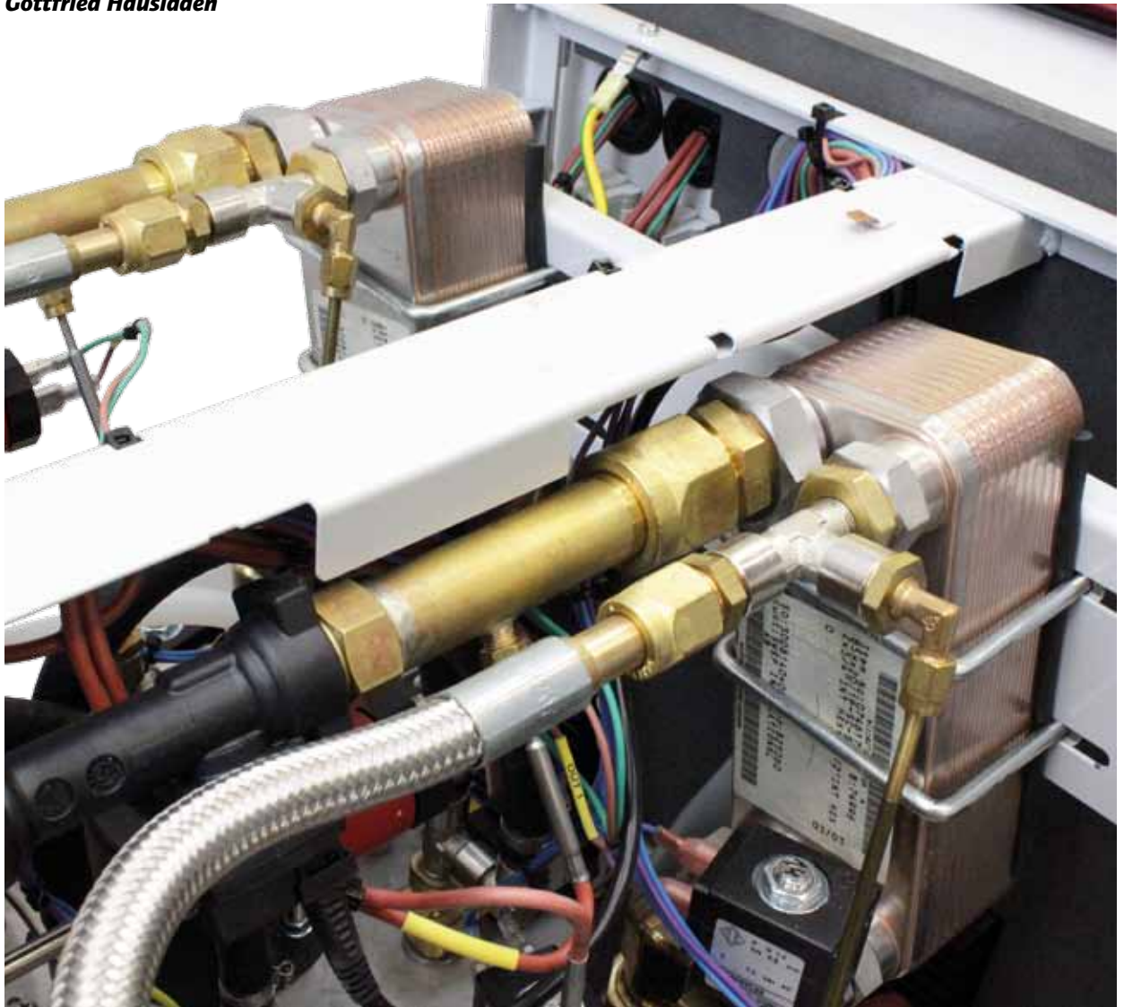
A view of the special technical equipment of the temperature controllers in operation at FKT shows the additional heat exchanger plates installed in the TEMPRO plus D appliance.
