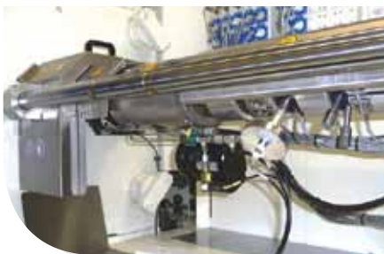
CELLMOULD®: Spritzeinheit/ injection unit
