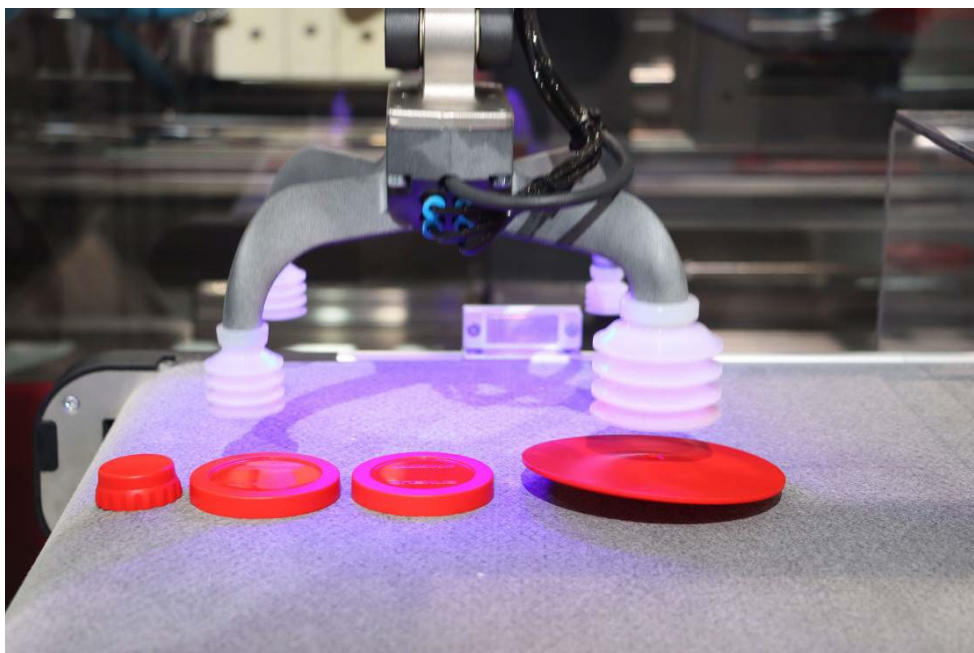
Fig. 2: LSR closing caps for beverage cans
