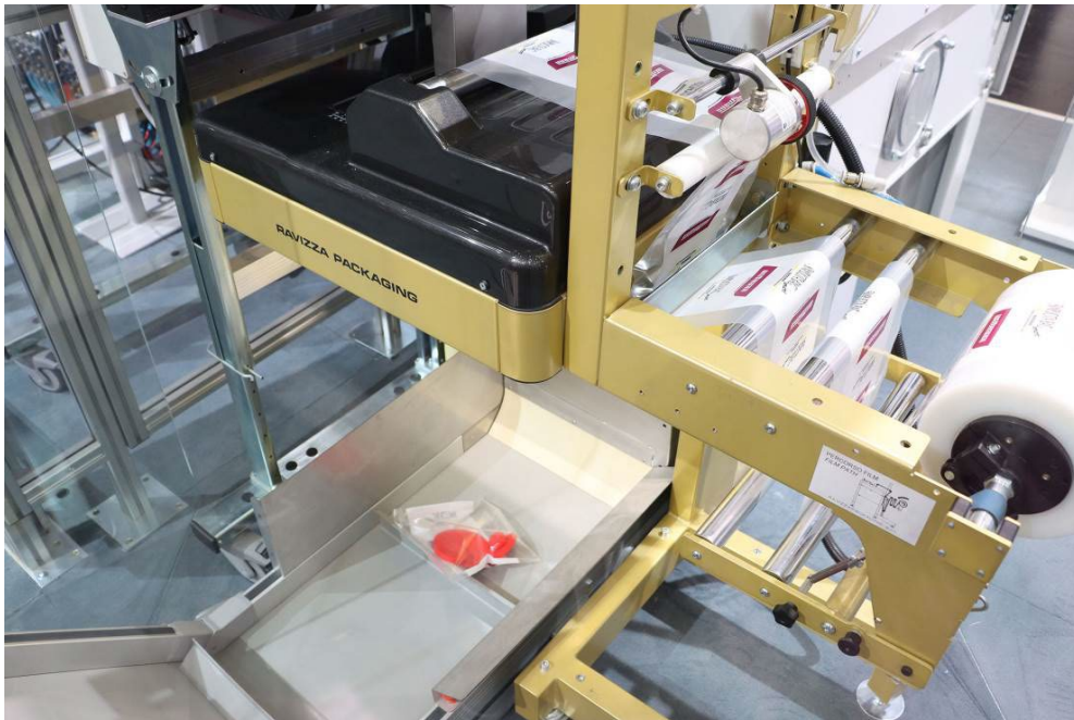
Fig. 3: Packaging of parts by a flow wrapping machine
