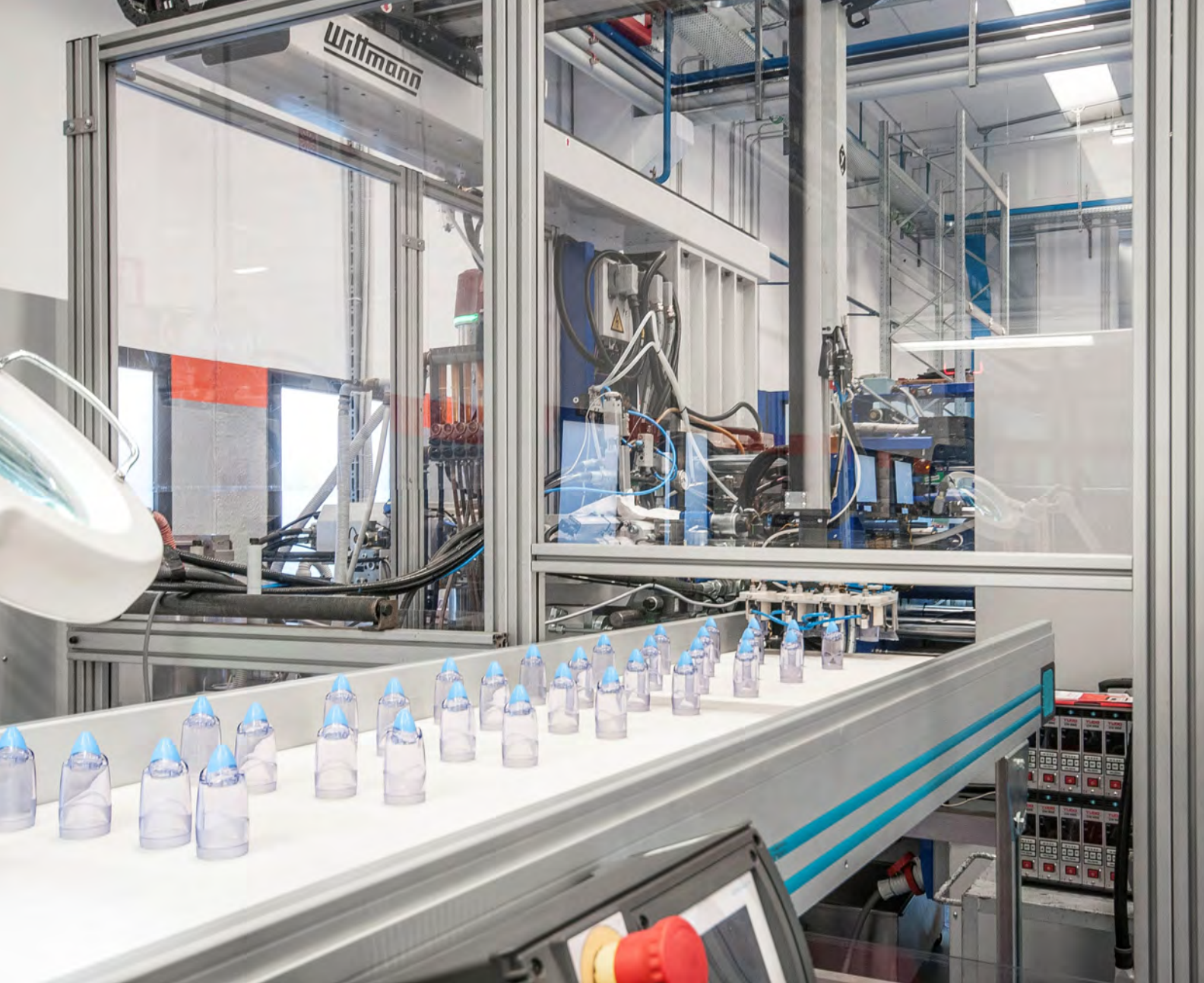
Oldrati has developed a molding process with one-shot technology for parts consisting of thermoplastics combined with silicone, including specially designed molds suitable for the necessary heating and cooling processes. This picture shows a working cell from the WITTMANN Group.
