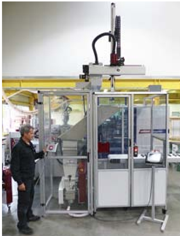
G-Max 12 within the protective housing of a working cell
