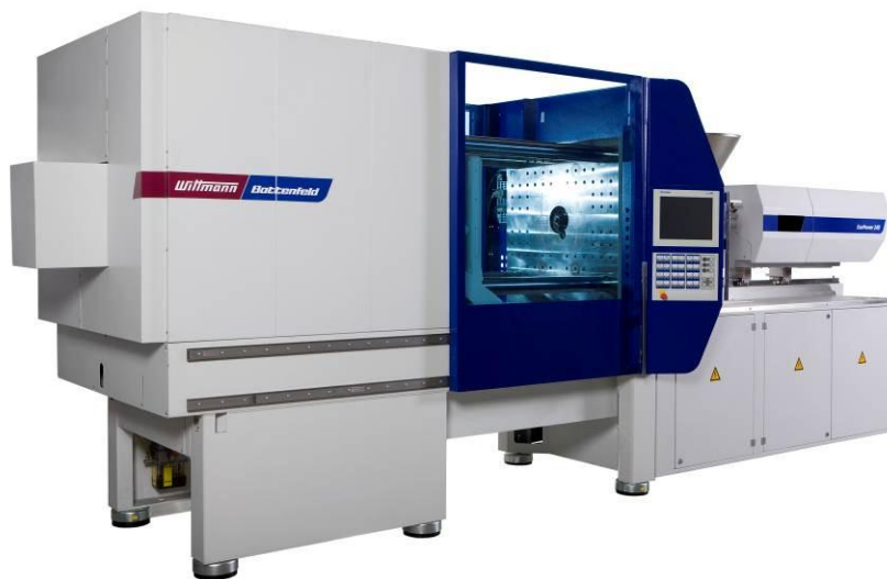
Fig. 1: The parts are produced on an EcoPower 240/1330 equipped with the HiP-Opening program and the Wittmann Battenfeld CELLMOULD® package
